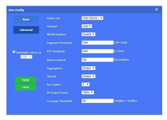
Channel: Auto in default, but recommend to setup channel by manual based on environment.
