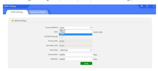
Static IP: Assign IP address and DNS information to get the Ethernet
