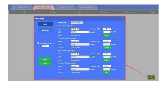
Wireless Basic: to setup wireless AP's SSID, password, Tag VLAN
