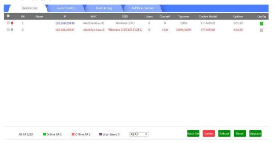
All AP: Show QTY of wireless AP which connected with this WLAN controller; 20 mean max to manage 20PCS wireless AP.
