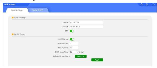
IP address: mean AC controller's IP address
