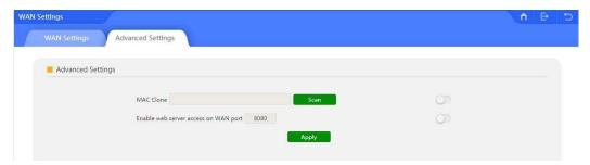
MAC Clone: When enable it, can scan the connected device's MAC address, choose the MAC address needed to be cloned, then apply; Or can input the indicated MAC to clone.
